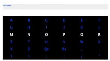
Figure 2 The P3S is a matrix of letters, where each row and each column are intensified and the intensifications are presented in a random sequence.
